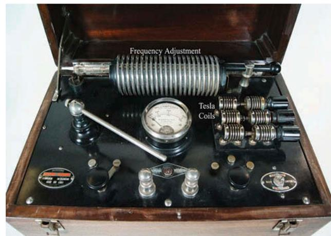
**Figure 2.** McIntosh diathermy with adjustable frequency and Tesla coils (From the collection of John Abele with kind permission of John Abele and Steven D Schwaitzberg).
