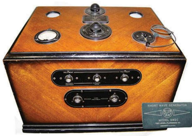
**Figure 4.** Liebel-Flarsheim short wave radiofrequency generator from the 1930s (From the collection of John Abele with kind permission of John Abele and Steven D. Schwartzberg).
